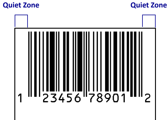
Figure 6 • Quiet Zone in a Bar Code
